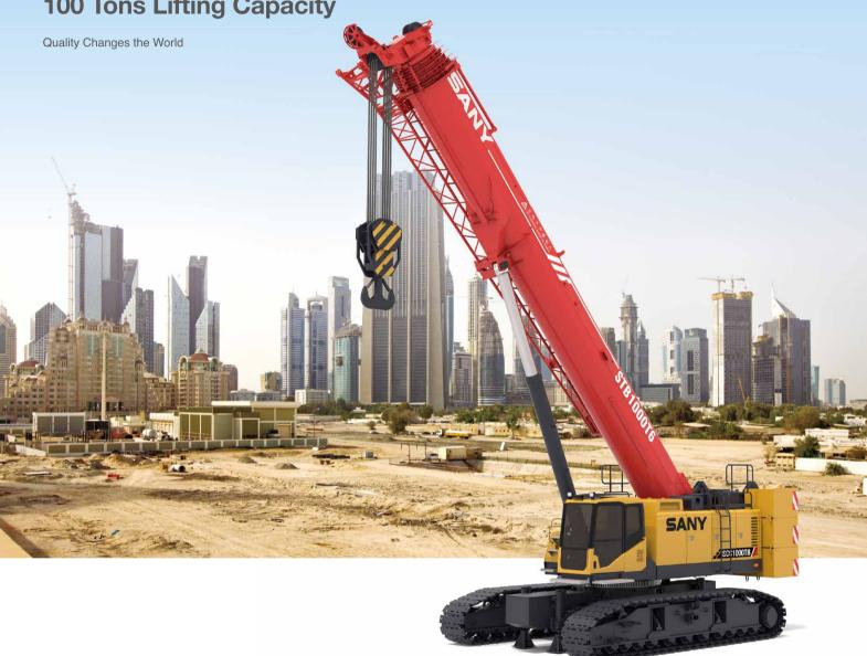
Max. lifting moment: 378t⋅m Max. boom length: 59m
