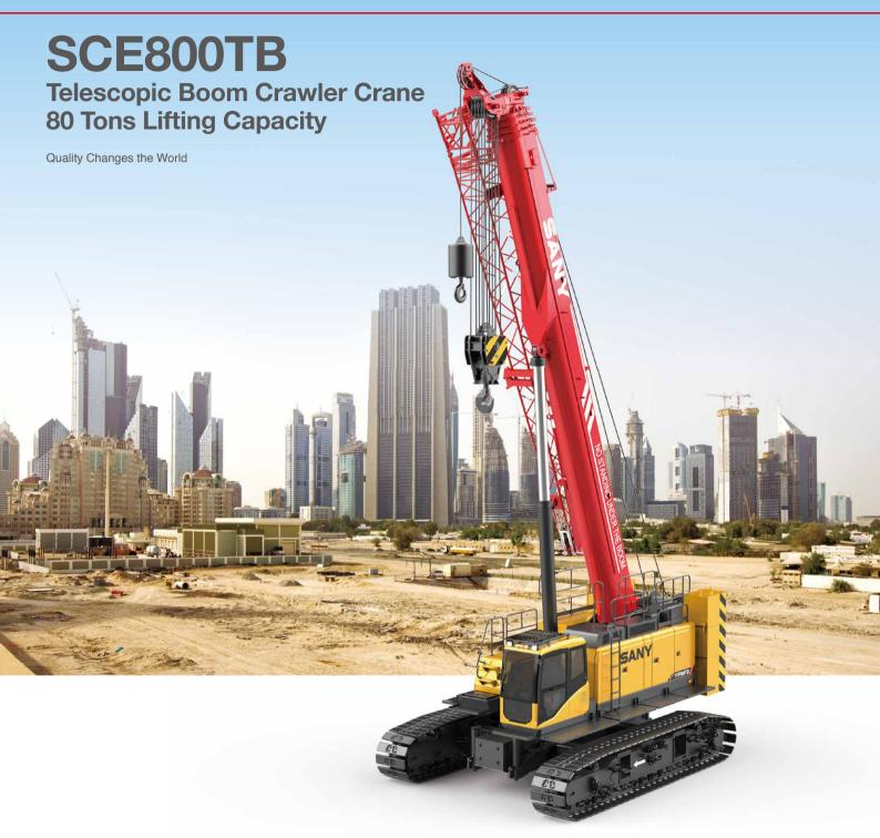
Max. lifting moment: 300t·m Max. boom length: 47m
