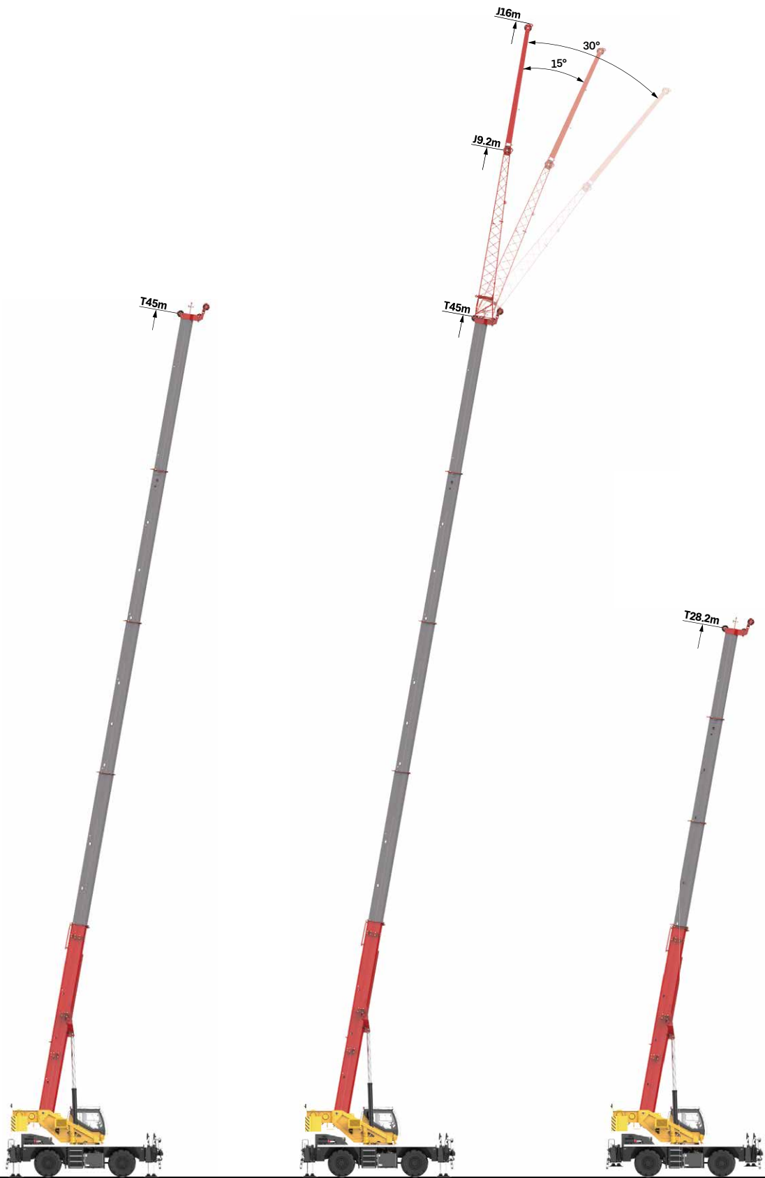
Telescopic boom on outriggers 主臂、支腿吊载
