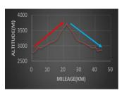
Average slope 5%, the energy recovered from full-load 80t downhill can cover the consumption of no-load uphill, and the energy consumption is 0 kWh/km.
