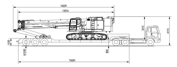
■ Transport mode 2: basic machine (without counterweight and hook) 41.3t + counterweight and hook transport 21.7t, a total of 2 truckloads.
