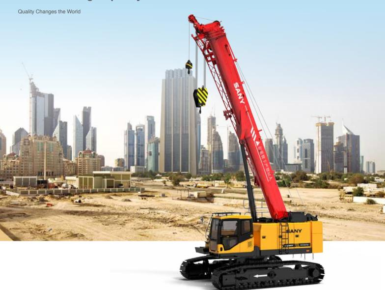
Max. lifting moment: 216 t⋅m Max. boom length: 42 m
