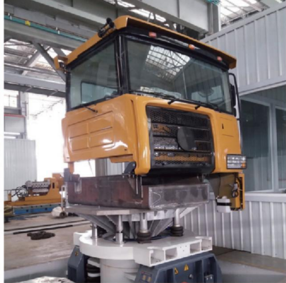
Cab shock test
