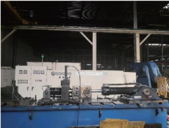
Front suspension cylinder durability test
