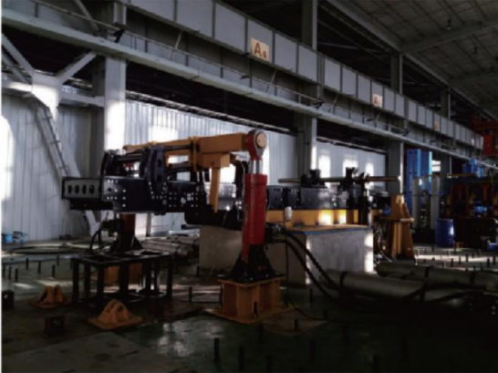
Frame fatigue test
