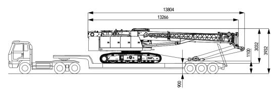
■ Transport mode 2: remove the counterweight and transport through two vehicles. The maximum weight of single piece transport is 29t, 13.26m×2.99m×3.03m (L×W×H)
