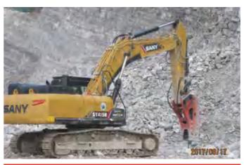
Worksite: Huzhou Tarmac Mining of Zhejiang Province Working condition: Stonework (decomposed rock) Operating type: excavation- loading Work undertaken by SY415: Stone stripping, and loading
