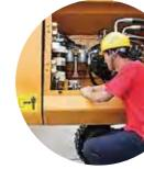
Replace diesel oil filter element
