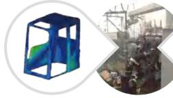
vibration test bench and test bed, fuel tank and the cab has been tested by over hundreds of thousands of times on aspect of the vibration to improve the service life of the component by 50%.
