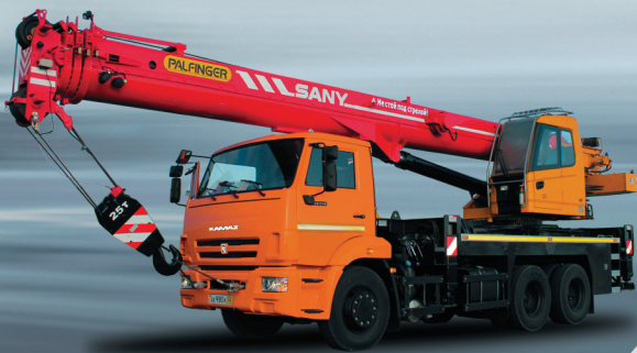
32 TONS TRUCK CRANE BOOM 10.2-32 m
