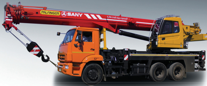
25 TONS TRUCK CRANE BOOM 10.2-32 m
