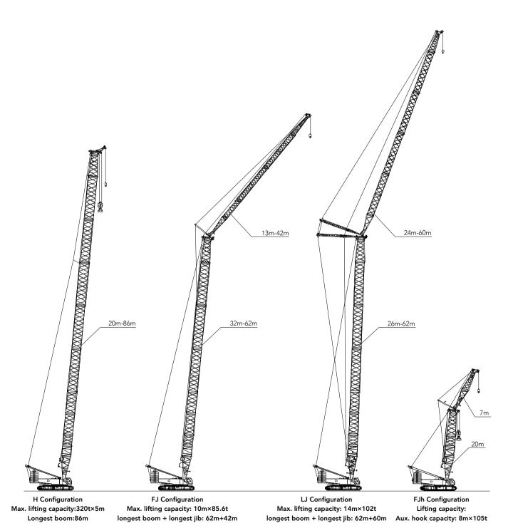
Main hook capacity: 10m×180t Boom combination: 20m+7m
