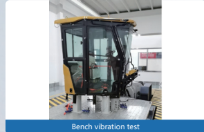
Bench vibration test
