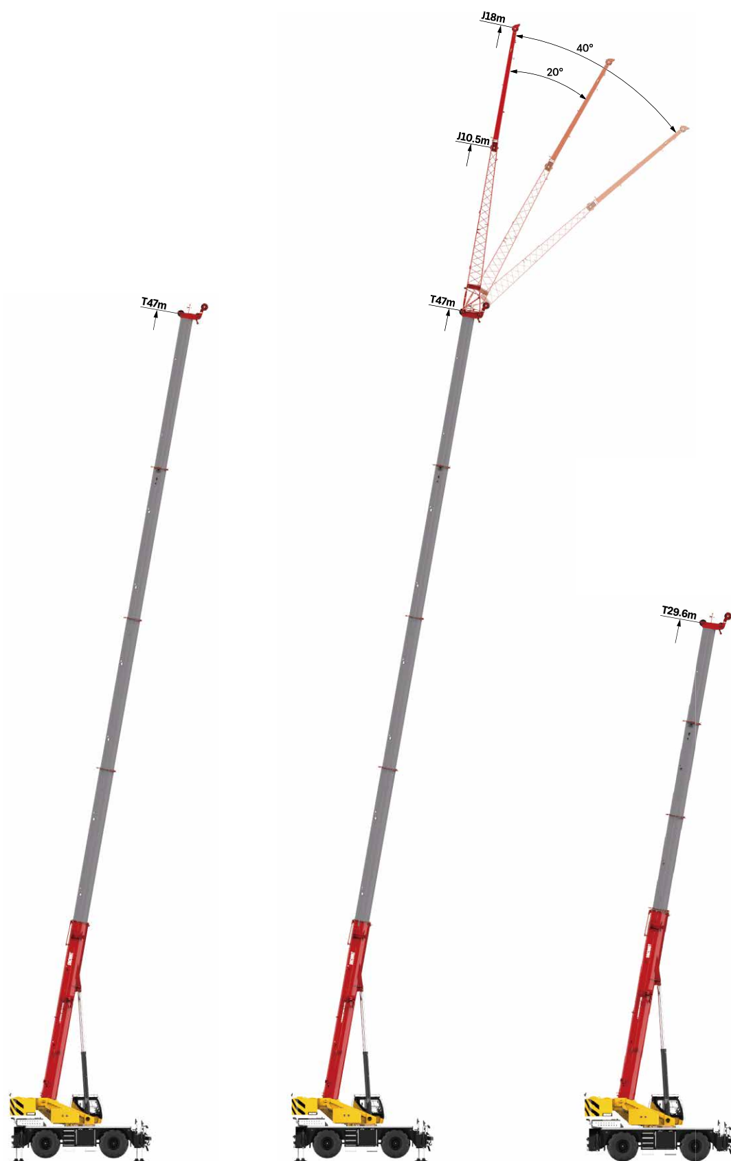
Telescopic boom on outriggers 主臂、支腿吊载
