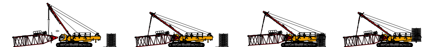
Self-assembly of boom base and 3m boom insert 主臂下节臂与3m主臂中间臂自装卸
